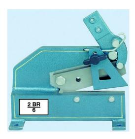
Table top metal shear design for cutting plate and round bar. Blades can be easily removed for sharpening or replacing Shear capacity bar 13mm Extension arm supplied
