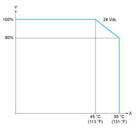
X: Ambient temperatureY: Input simultaneous ON ratio
