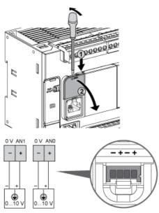
The (-) poles are connected internally.
