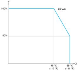
X : Ambient temperature Y : Input simultaneous ON ratio
