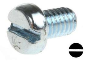
Cheese Head Machine Screws are designed for ease of assembly and these screws with their slotted drives are a popular driving method with this type of fastener. Machine screws can be used in pre-tapped holes or used with conforming nuts and washers in through-holes.
