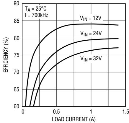
**Efficiency,  $V_{OUT} = 1.8V$**
