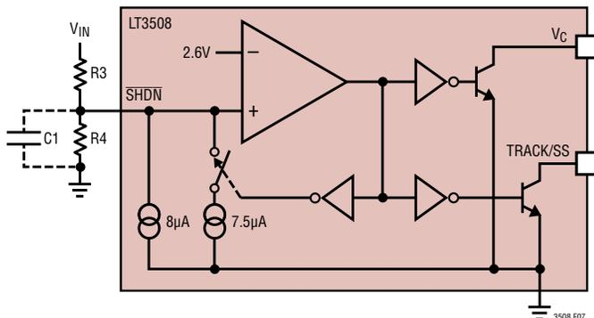
Figure 7. Undervoltage Lockout
