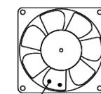
**Note:** The glues on the impeller is for impeller balance. Do not remove it.
