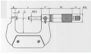
Outside Micrometer 0-1" Accuracy: 0.004mm A: 3.0mm B: 6nm C: 24mm D: 32mm Outside Micrometer 1-2" Accuracy: 0.004mm A: 3.0mm B: 8mm C: 32mm D: 57mm Outside Micrometer 2-3" Accuracy: 0.004mm A: 3.0mm B: 8mm C: 45mm D: 82mm Outside Micrometer 3-4" Accuracy: 0.005mm A: 3.0mm B: 8mm C: 57mm D: 107mm Accuracy: 0.006mm A: 30mm B: 6mm C: 70mm D: 133mm Outside 4-5" Micrometer Outside Micrometer 5-6" Accuracy: 0.006mm A: 3.0mm B: 6mm C: 82mm D: 158mm
