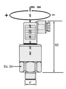
F4 adjustable pressure switches provide an electrical signal once a set pressure value is reached. Pre-set pressure is adjusted by rotating a screw, located in the centre of the switch, clockwise to increase pressure & anti-clockwise to decrease pressure.
