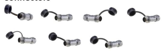
The RS PRO ST12 series is a range of small but robust waterproof connectors, which are sealed to IP67. Threaded coupling ensures a secure connection, and black nickel-plated zinc alloy bodies provide an attractive finish. Versions are available for in-line cable to cable and for cable to panel connections. Plugs and receptacles are available with either male pins or female sockets.
