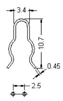
Mounting Hole Hole in PCB φ0.8 to φ1
