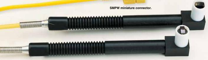
Model No. 88102(\*) Right-angle, pencil-type surface probe, best suited to stationary surfaces. Sensing element is perpendicular to the handle 250°C (480°F) max surface temperature.
