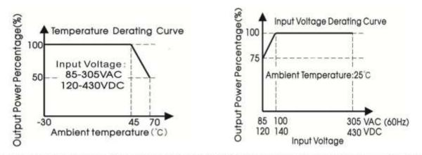
Note: 12With an input voltage between 85-100VAC and a DC input between 120-140VDC, the output power must be derated as per the temperature derating curves:
