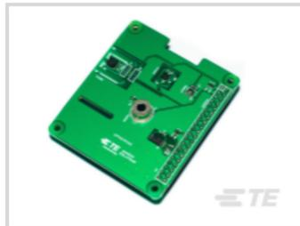
Digital Component Sensor Product Type: **Shield for Raspberry Pi**
