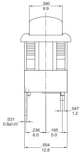
Dimensions : Inches/Millimetres Tolerances ±0.012"/0.3mm
