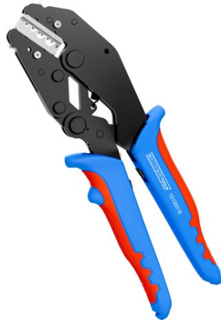
ERGO-CRIMP was developed for the process-safe crimping of various electrical connectors. The crimping tool has a ratchet mechanism with a blocking device to ensure a consistently high crimping quality and results that can be precisely repeated. The mechanism only opens the tool when the crimping process is complete. In addition, an emergency release has been integrated into the handle, which allows the user to open the crimping tool whenever necessary, e.g. in the event of misuse.
