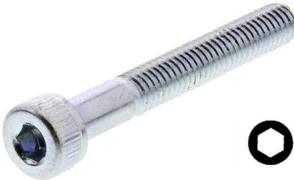
Socket Caps have a small cylindrical head with tall, vertical sides giving them space saving advantages as well as greater tensile strength. They also require less side room for wrenches. These socket screws are used in many applications including the manufacture and repair of vehicles, machine tooling, tools and dies, machine production and repair and general engineering applications. Most importantly, socket cap head screws provide safety, reliability and cost efficiency.
