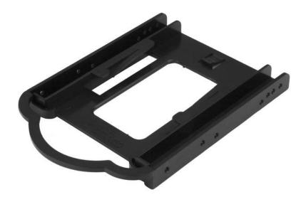
The 2.5" SDD / HDD Mounting Bracket for 3.5 Drive Bay now comes in a convenient 5-pack. This mounting bracket lets you quickly install a 2.5" SSD or HDD into a single 3.5" bay in a desktop PC or server, with no tools required. The tool-less mounting bracket supports a 2.5" solid-state drive or hard drive from 7 mm to 9.5 mm in height.
