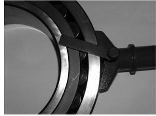
The inner ring holders must be placed on the same side of the bearing. Make sure that the inner ring holders are not placed in the bore of the inner ring or against the cage or rollers. Placing the inner ring holders incorrectly will damage the bearing or make the bearing difficult to mount on the shaft.
