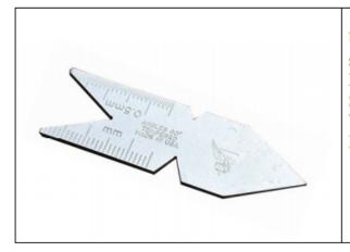
Used for checking 60 degree tool points and setting screw thread cutting tools Manufactured from tempered steel Satin chrome finish Working surfaces are ground for accuracy Both sides marked with 0.5 and 1mm graduations
