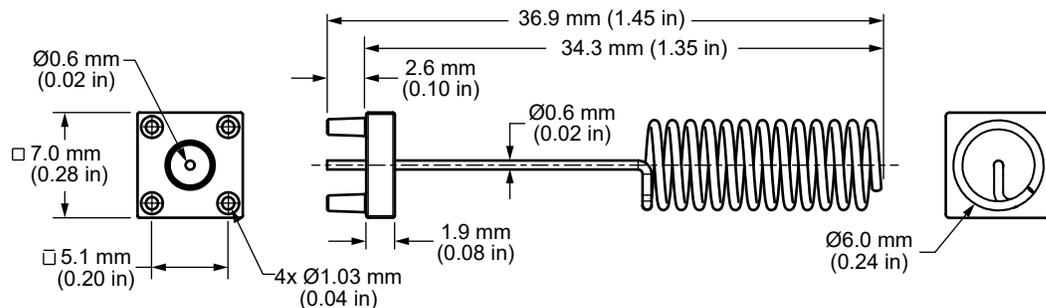
Figure 1. ANT-2.4-VHETH Antenna Dimensions
