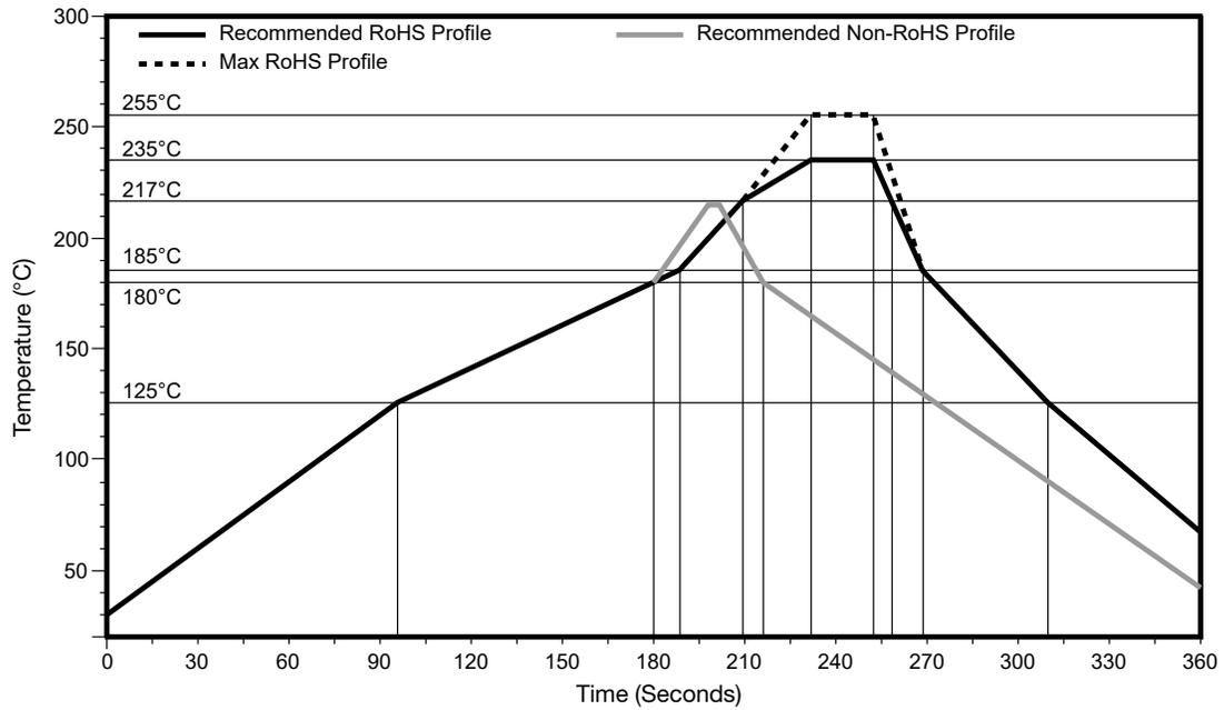
Figure 11. Solder Profile for the ANT-868-VHETH Antenna
