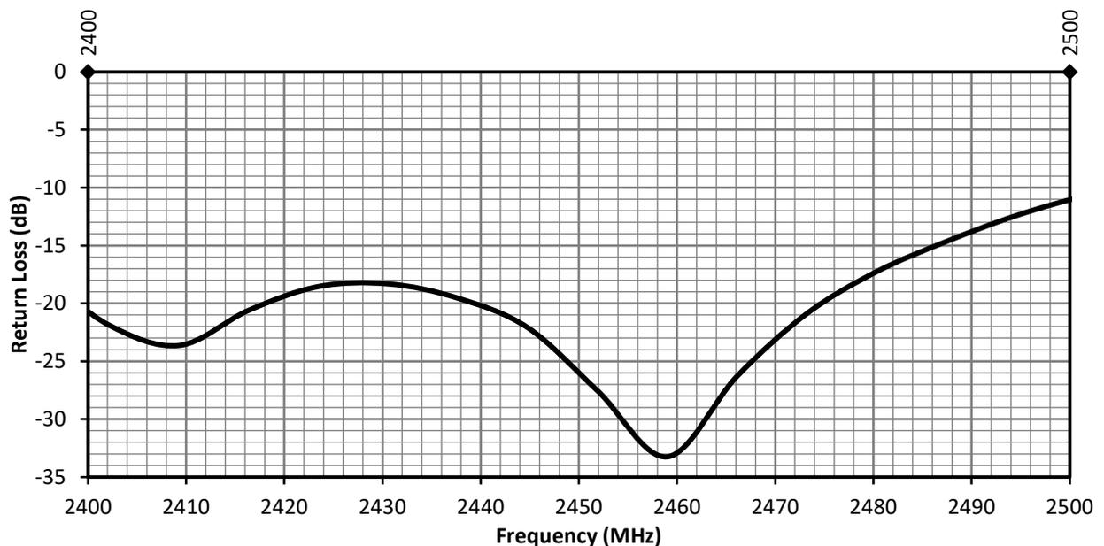
Figure 3. ANT-2.4-VHETH Antenna Return Loss
