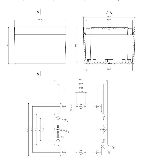
Dashed line shows outline of the mounting boss under PCB board Recommended mounting holes diameter Ø4mm
