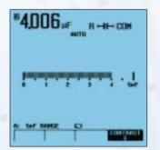
Check the starting capacitor of a motor with the ScopeMeter 123
