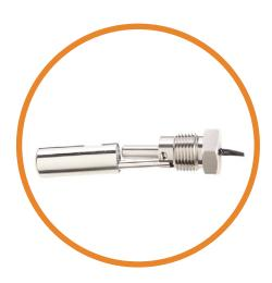
This flat switch is horizontally mounted switches that are fitted via a 1/2"NPT thread from the outside of the tank, so does not require access to the inside of the tank.
