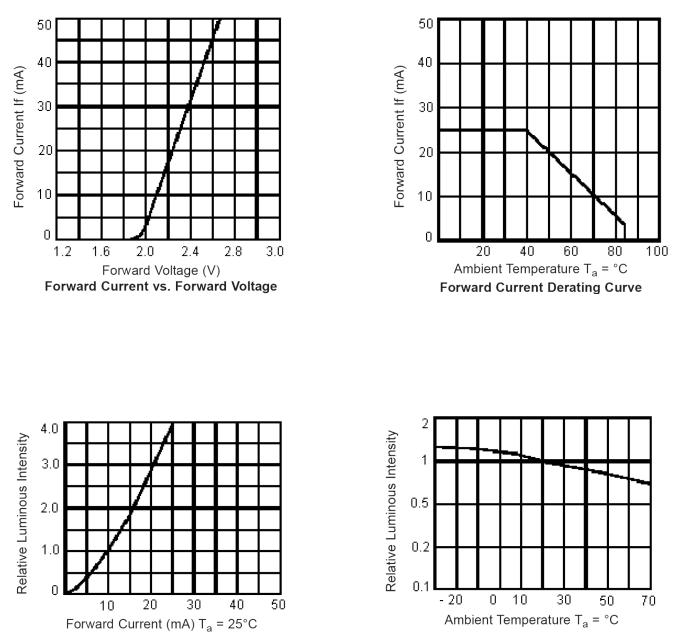
Luminous Intensity vs. Forward Current
