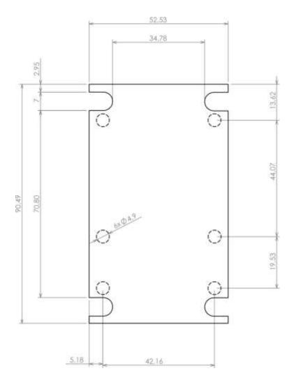
Dashed line shows outline of the mounting boss under PCB board Recommended mounting holes diameter Ø3,5mm All dimensions are given within +/-0,5mm tolerance
