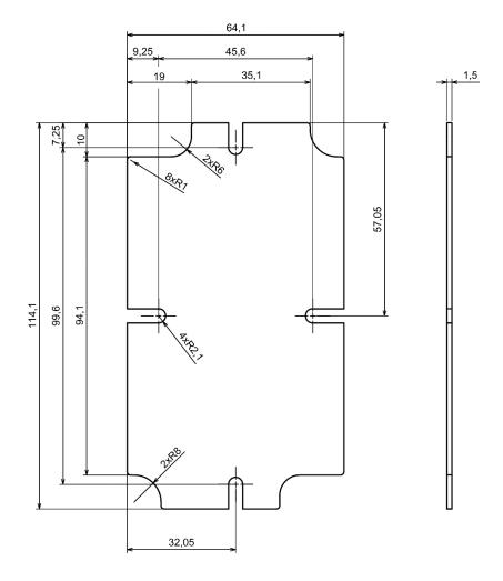
All dimensions are given within +/-0,5mm tolerance
