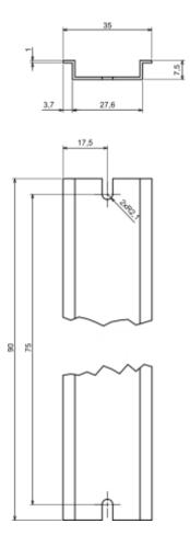
All dimensions are given within +/-0,5mm tolerance
