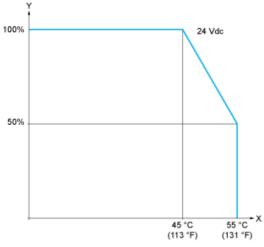
X: Ambient temperatureY: Input simultaneous ON ratio
