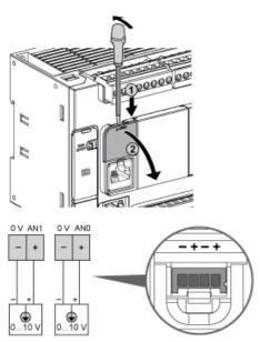
The (-) poles are connected internally.
