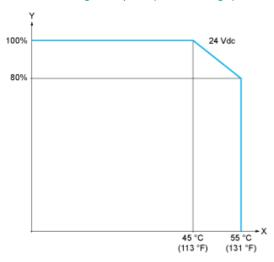
X: Ambient temperatureY: Input simultaneous ON ratio
