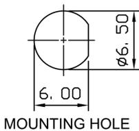
1. IP67 SMA B/H Jack for OD1.37mm Cable
