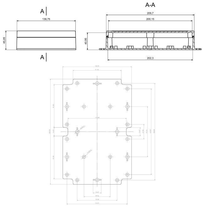
Dashed line shows outline of the mounting boss under PCB board Recommended mounting holes diameter Ø4mm
