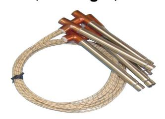
Air heaters feature an open coil of high temperature resistance wire electrically isolated in a stainless steel sheath. Because the air being heated passes directly over the resistance wire, maximum heat transfer efficiency is achieved. Ar heaters are used for heat staking, plastic welding, laminating, drying, heat sealing, and any other operation where air needs to be heated up 500°C
