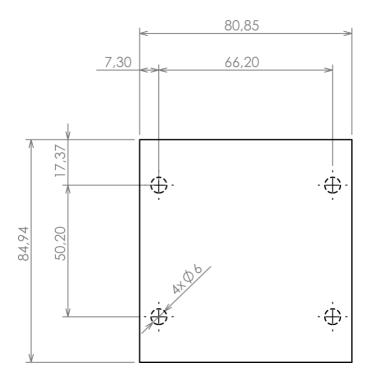
Dashed line shows outline of the mounting boss under PCB board Recommended mounting holes diameter ø3,5mm
