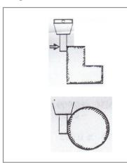
Test the Edge Finder before use with a conductive metal wire or flexible steel rule to ensure it illuminates when a circuit is made between the probe and the main shaft
