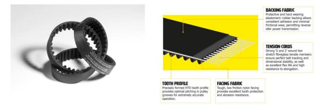
RS Pro HTD Timing belts can be used in drive system applications. High power transmission via its unique tooth profile, enables it to be used in low speed, high torque applications.
