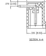
Positions: 02 thru 24 A = .197 [5.00] x No. of Positions+ .055 [1.40] B = .197 [5.00] x No. of Spaces
