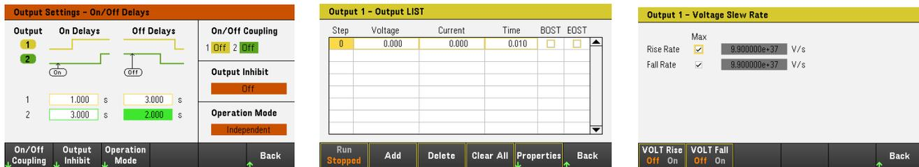
Figure 8. Output sequencing and output LIST mode, with slew rate setting
