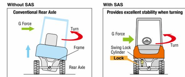
An onboard computer monitors the movement of the forklift and locks the swing of the rear axle when necessary, such as during turns.
