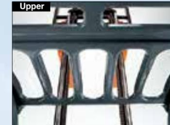
The overhead guard, mast and instrument panel have been designed to provide excellent visibility of the fork tips at the most frequently used lift heights.
