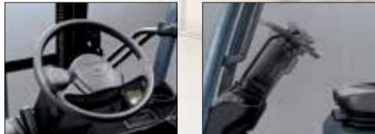
The small-diameter steering wheel teams up with the full hydraulic power steering system to provide excellent maneuverability. The steering column offers step-less adjustment to accommodate a wide range of operator preferences.
