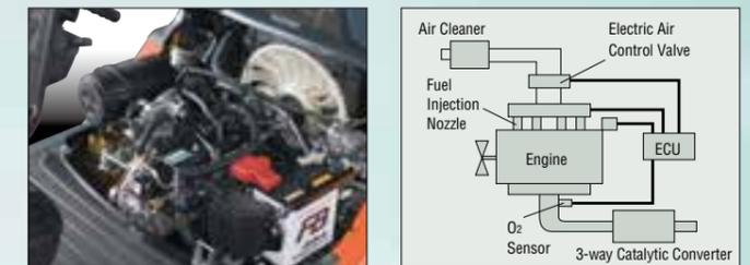
Electronic control is used on the 4Y engine to regulate the fuel injection and ignition systems. This is combined with the 3-Way Catalytic Converter System to filter out carbon monoxide (CO), hydrocarbon (HC) and nitrogen oxide (NOx) gases.
