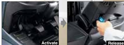
The operator simply depresses the parking brake pedal to set it without changing operating position. A conveniently located handle is used to release it.
