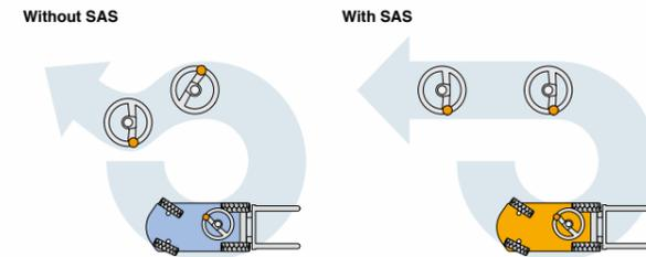
This function ensures that the angle of the steering wheel corresponds to the angle of the rear steered wheels.
