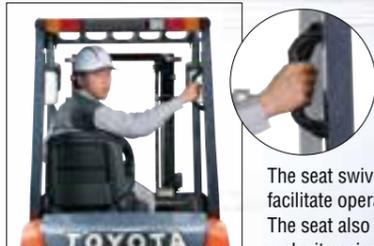
The seat swivels to the right to facilitate operation in reverse. The seat also swivels to the left to make it easier to enter and exit
