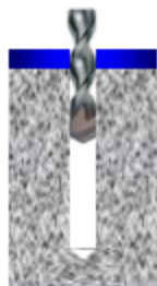
Position fixture and drill correct diameter hole to correct depth
