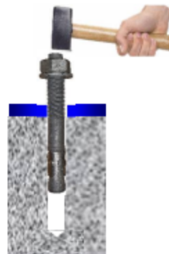
Insert assembled anchor through fixture into concrete
