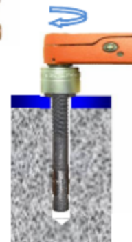
Tighten with torque wrench to Installation Torque
