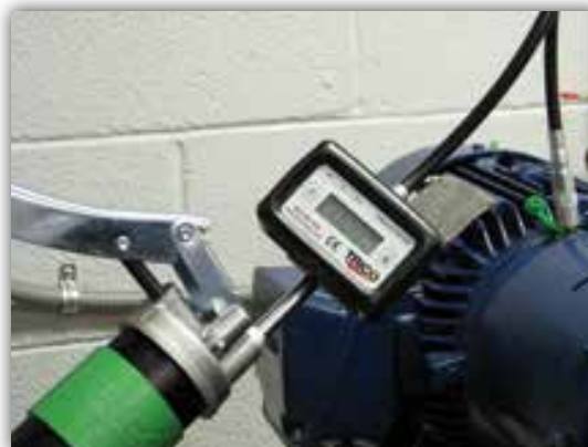
Grease meter being used with Spectrum Grease Identification Products to ensure the right grease goes into the right piece of equipment.
