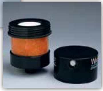
The reusable top cap contains the inlet and outlet valves which protect the silica gel from excess humidity.
