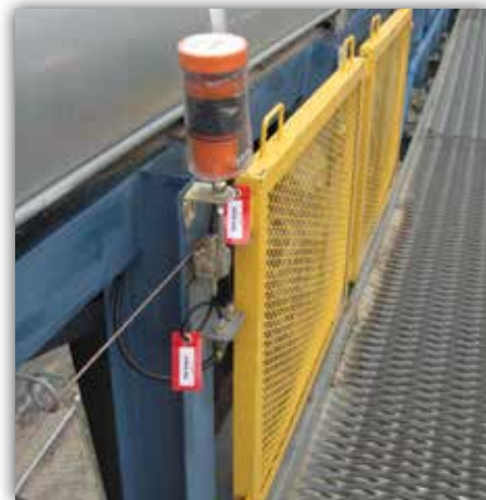
Spectrum Tags and Labels are used to identify grease lines for Automatic Grease Dispensers.
