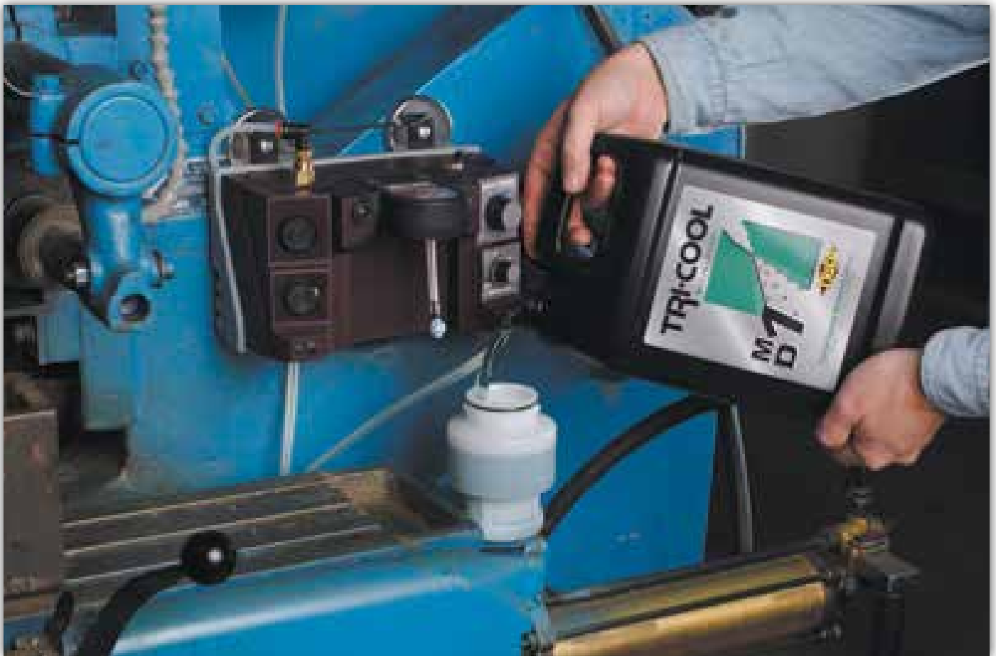
Micro-dispenser being filled with Tri-Cool MD-1 lubricant
