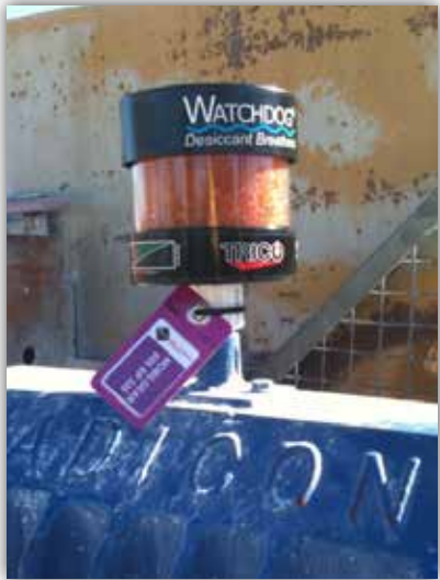
Spectrum Tag on a Watchdog Desiccant Breather
