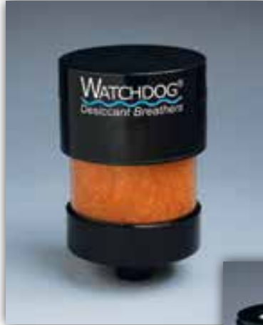
The reusable top cap with inlet and outlet valves allows the economic replacement of the desiccant cartridge.
