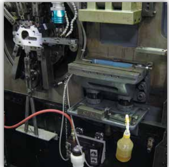
Minimum quantity lubrication used on a tapping workcenter
