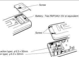
Fuse : F 600V/10A (Fast action type)  $\phi$  6.3 x 32mm F 600V/500mA (Fast action type)  $\phi$  6.3 x 32mm —
