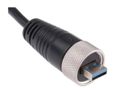
The RS PRO series of waterproof metal USB-A connectors are a range of ruggedised IP67/IP68 connectors designed to be used outdoors or in harsher industrial environments. Designed to fit panel cut outs of 25.5mm the metal USB-A series also comes with rear potting on the panel mount connectors. This ensures your panel is still sealed to an IP67/IP68 rating even when the connector is unmated, and the sealing cap is not connected. The threaded mating allows for a secure connection.
