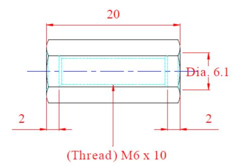
Material : Cold Rolled Steel. Finish : Zinc Plated
