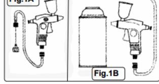
3.6. Ensure the valve is turned fully anti-clockwise before screwing to the top of the propellant can, fig.1.B.
