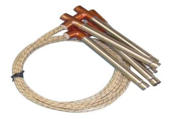
Air heaters feature an open coil of high temperature resistance wire electrically isolated in a stainless steel sheath. Because the air being heated passes directly over the resistance wire, maximum heat transfer efficiency is achieved. Ar heaters are used for heat staking, plastic welding, laminating, drying, heat sealing, and any other operation where air needs to be heated up 500°C
