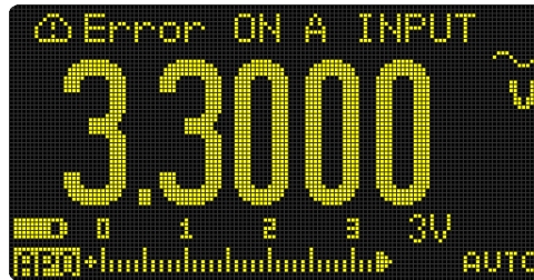
Figure 1-3 Input warning display (A INPUT)
