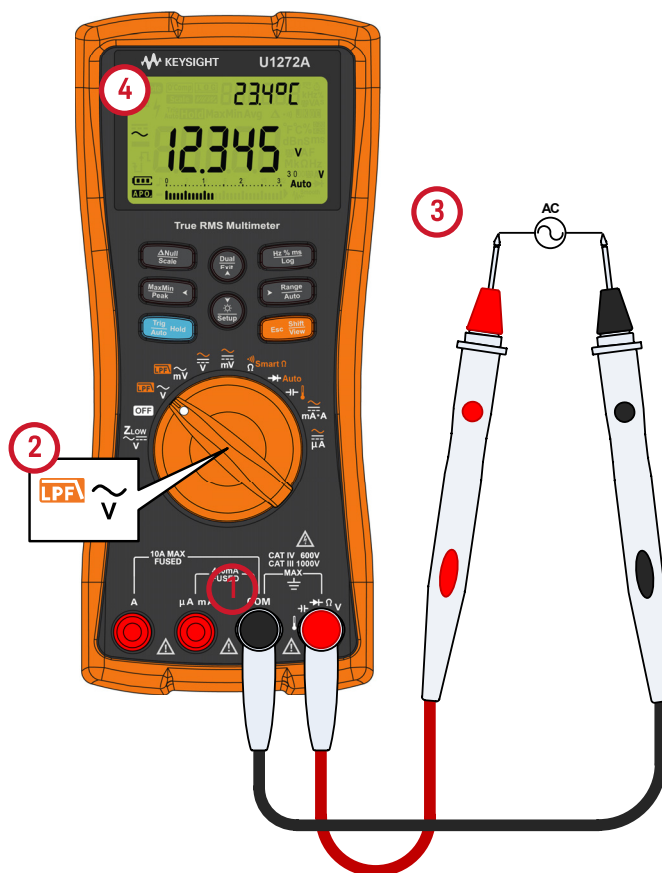
Figure 2-2 Measuring AC voltage
