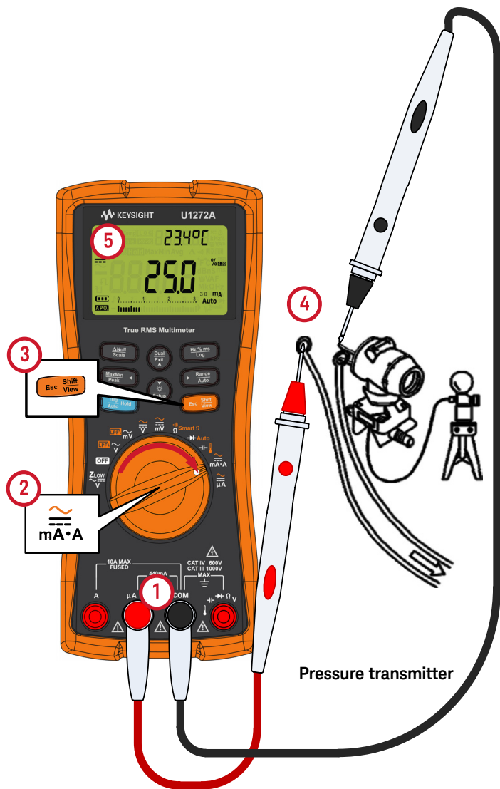
Figure 2-36 Measuring DC current using the 0-20 mA % scale
