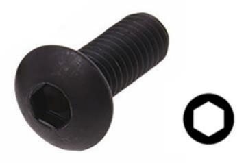
Button Head Socket Screws are designed for light duty. They have a similar thread design as a Socket Cap Screw although the dome-shaped head is wider and has a lower profile than a Socket Cap Screw, presenting an aesthetic appearance in an assembly. These fasteners are ideal when a wider bearing surface is required.
