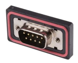
The RS PRO series of waterproof D-sub connectors are a range of ruggedised IP67 connectors designed to be used outdoors or in harsher industrial environments. Designed to fit panel cut outs of 40.0mm the waterproof D-sub series also comes with rear potting on the panel mount connectors. This ensures your panel is still sealed to an IP67 rating even when the connector is unmated. The Push-Fit with dual Screws mating allows for a secure connection.
