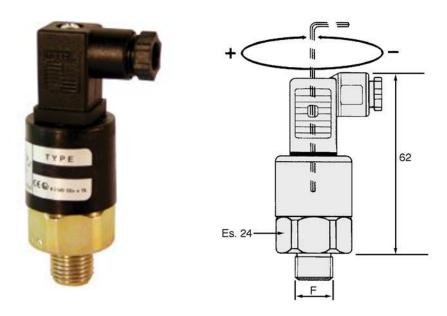
F4 adjustable pressure switches provide an electrical signal once a set pressure value is reached. Pre-set pressure is adjusted by rotating a screw, located in the centre of the switch, clockwise to increase pressure & anti-clockwise to decrease pressure.
