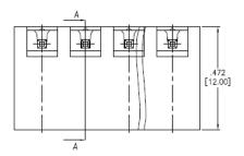
Positions: 02 thru 24 A = .200 [5.08] x No. of Positions+ .055 [1.40] B = .200 [5.08] x No. of Spaces
