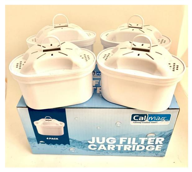
Hard water cartridge – silver impregnated coconut activated carbon effectively reduces organic contaminants, chlorine, trichloromethane and insecticides. Sodium-less ion exchange resin reduces inorganic contaminants, lead, copper and limescale.
