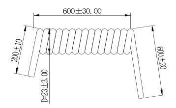
Cable Marking: RS PRO 2x0.75mm<sup>2</sup> Coiled Power Cable 300/500V
